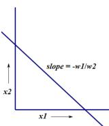
A perceptron is a binary classifier when the two classes can be separated by a straight line.
