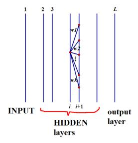
To use GRADIENT DESCENT, we have to make sure that the output from every node is continuous.
